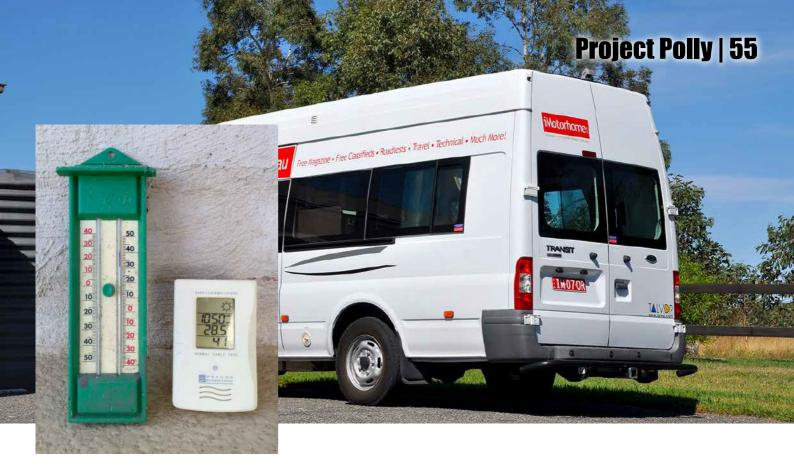
**Insert:** Shade air temperature was averaged from the readings of these two thermometers plus a nearby Bureau of Meteorology weather station. **Above:** With the screens removed the interior temperature rose much more rapidly and was nudging 50°C at 2 pm when storms arrived. Winter heat loss would be just as dramatic.
